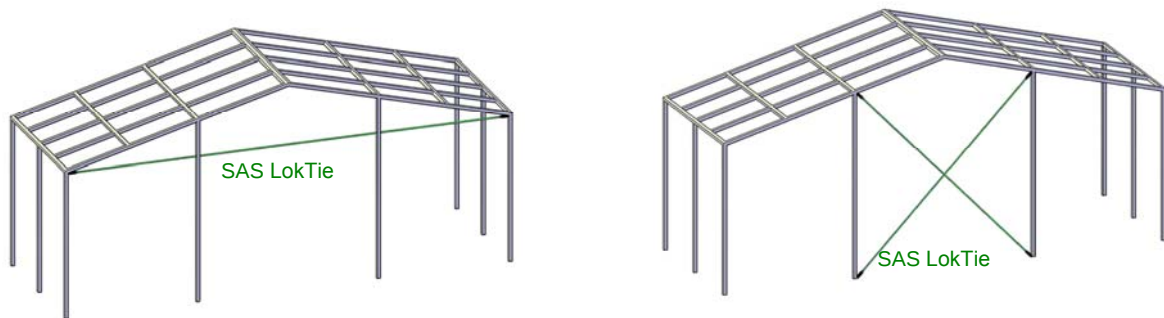
Fig. 3: Example: an application of SAS LokTie in industrial facilities.
