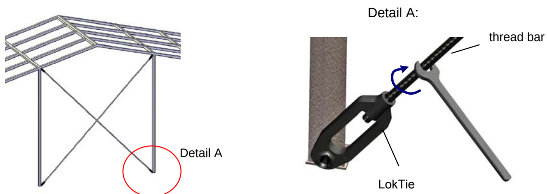
Fig. 4: Construction of the LokTie
